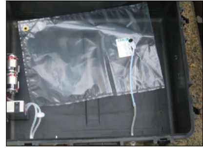
Photo 14-1: Vacuum chamber and Tedlar bag © CH2M HILL
