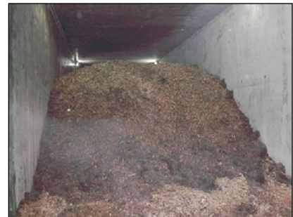
Photo 5-19: Aerated static pile composting inside an enclosed concrete tunnel © Scott Gamble
