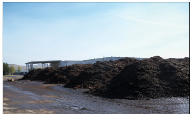
Photo 3-3: Windrows are commonly used for curing © CH2M HILL
