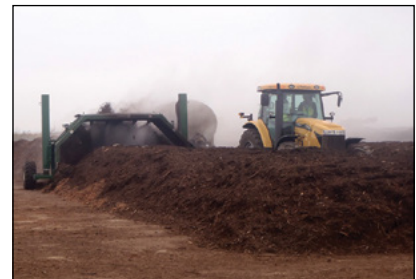
Photo 5-8: Typical windrow operation with a towed windrow turner © CH2M HILL
