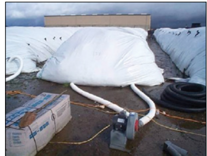
Photo 5-14: Composting system using polyethylene covers © Scott Gamble
