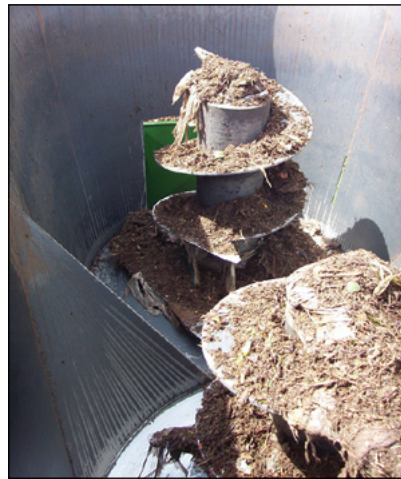
Photo 11-4: Augers inside a vertical mixer © Scott Gamble
