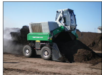
Photo 5-7: Straddle-style windrow turner © CH2M HILL
