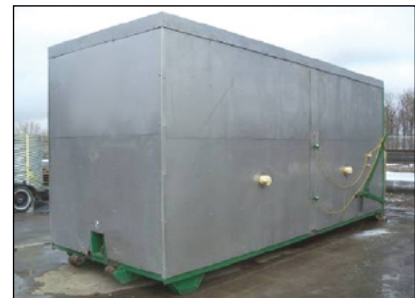
Photo 5-20: Static container composting system © CH2M HILL
