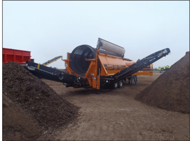
Photo 11-7: Trommel screen: Oversize materials fall from the drum onto the left conveyor, and fine materials fall through the screen and are discharged off the conveyor to the right © CH2M HILL
